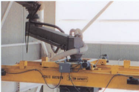
Articulating Arm accepts materials from fluidized conveyor.
