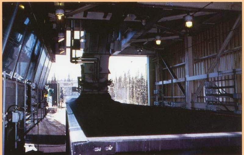
Because the material is dropping only a short distance from the gate at the chute bottom to the car, dusting is dramatically reduced.
