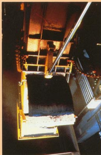
At the operator's command, this gate activates from fully closed to fully open in seconds, giving pinpoint control to the operator.
